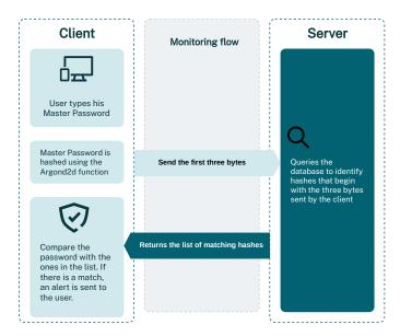
Figure 6: Dark Web monitoring for Master Password flow
