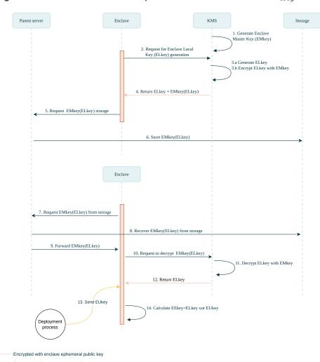
Figure 14 describes the workflow to provide secure enclaves with  $EL_{Key}$ .
